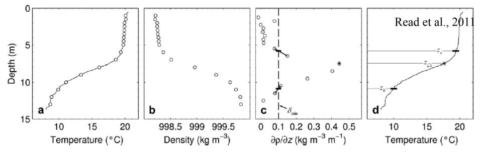
Can be used to calculate the depth of each of the three main vertical layers of lakes
